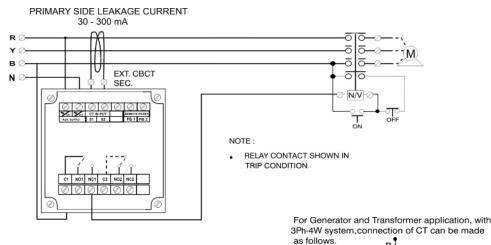
Earth Leakage Monitoring of 3 Phase System, Microcontroller based design, Manual / Remote Reset, Sensing 30 - 300 mA Primary Leakage Current, Input through CBCT, Adjustable Trip Settings, Adjustable Trip Delay, 2 CO Relay Output Contacts, Non -Fail safe Relay Output Logic.
