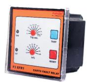
F3 EFR1 operates on current sensing principle and is used in electrical circuits & systems where EARTH FAULT protection is required. F3 EFR1 relay is more accurate, easy to set, compact and easy to install at panel facia .This relay offers ( 1CO/2CO) relay contact of 5Amps at 240VAC rating.
