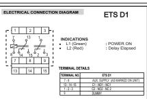
AUX. SUPPLY TO BE CONNECTED AS MENTIONED ON THE UNIT ■ RELAY CONTACTS SHOWN FOR DELAY ELAPSED CONDITION.
