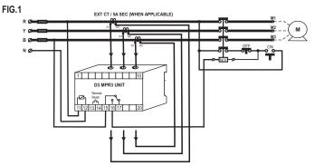
NOTE:- 1) EXTERNAL CT OF SEC 5A TO BE CONNECTED IN POWER WIRING WHEN RATED CURRENT > 100A 2) RELAY CONTACTS SHOWN FOR UNIT IN POWER OFF / TRIP CONDITION.
