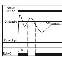
Power on Delay  $3.5 \pm 1.5$  Sec. (Fixed) Trip Delay set to minimum (i.e. instantaneous)
