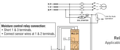
Relay contact Applicable for suction Tank
